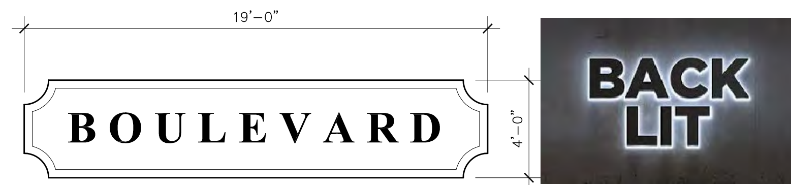
BUILDING PROJECTING SIGN AT BREEZEWAY (PHASE 2)
